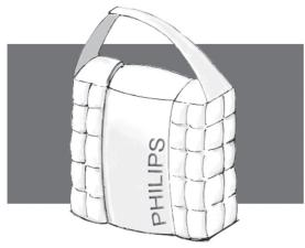
Figure 2 Inflatable packaging concept
